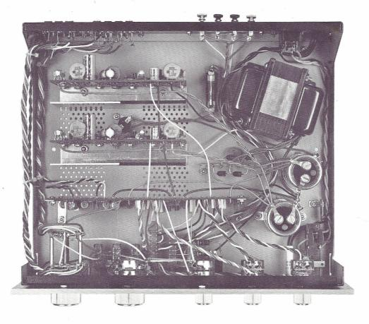
This photo shows the unit with the cover off. Notice the clean, uncluttered layout. Even the beginning audiophile can follow Dynaco's famous step-by-step kit instructions, once the technique of soldering is learned (a short course in how to solder is included, too). Seven wire colors and a single larger than life pictorial diagram, in color, indicate the connection and location of every component and wire, to make the SCA-50 simple, fun and easy to build.
